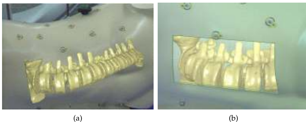
Figure 2.6: (a) and (b) show the overlay of the bone model and body surface with and without using the depth cue - occlusion Sources: images are taken from [4]
